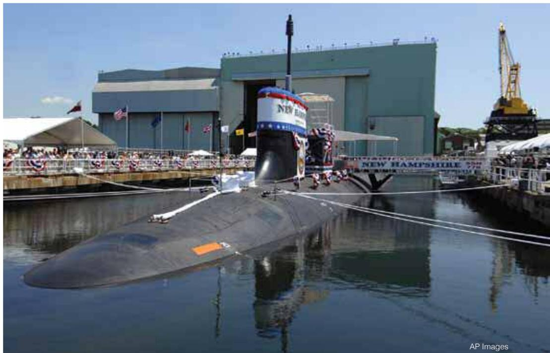
**The USS New Hampshire**, shown here at the General Dynamics Electric Boat Division in Groton, Connecticut, is one of 30 nuclear-powered attack submarines planned for the Navy at a cost of \$1.8 billion each.
